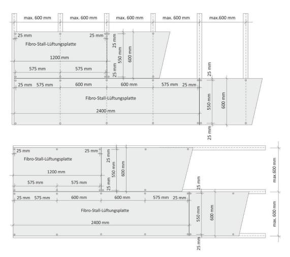
for board sizes: 2400 x 600 mm, or 1200 x 600 mm on wooden slat sub-structures or CD profiles
